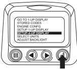
4. Touch the "Enter Button" to activate the "Use Defaults" function. This action will reset the unit to the factory default.
